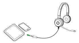
**NOTE:** When plugged directly into a mobile device, the overall call quality (for you and the listener) will be lower than when connected to a PC/tablet using the controller (Jabra Evolve Link).
