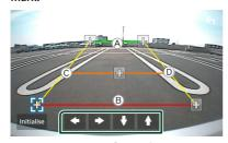
Make sure that lines (A) and (B) are horizontally parallel, and that lines (C) and (D) are of the same length.
