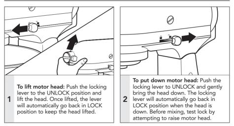
NOTE: Motor head should always be in LOCK position when using the Stand Mixer.
