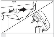
2 Hold the locking lever in the UNLOCK position and tilt motor head back.
