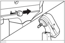
Hold the locking lever in the UNLOCK 2 position and tilt motor head back.
