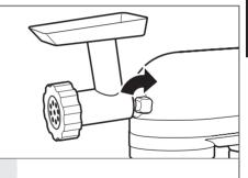
4 Tighten attachment knob by turning clockwise until attachment is completely secured to Stand Mixer.
