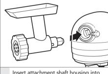
Insert attachment shaft housing into attachment hub, making certain that attachment power shaft fits into square attachment hub socket. It may be necessary to rotate attachment back and forth. When attachment
