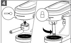
Position the Portafilter under the Group Head with the handle align to unlock. Raise the Portafilter into the Group Head and twist to the right side to lock.
