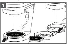
When the Drip Tray Indicator rises and becomes visible above the surface of the Drip Tray Plate, empty the Drip Tray and rinse with warm water.
