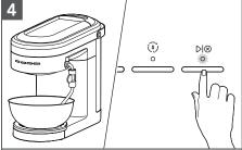
Phase 3: Place the container (~0.5 L) below the Steam Wand. Empty, rinse and refill the Water Tank with fresh water to Max fill line. Replace the Water Tank. Press ▶I⊗ button. Start/Cancel (▶I⊗) will blink fast after the third phase is complete. Empty the container.
