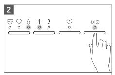
To change pre-programmed Water Volume for 1 / 2: Toggle the Mode Button to select Water. Select the dose you desire to programme (1 or 2). Press and hold ▶|⊗ button until desired water amount is reached in your cup.
