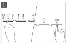
To change pre-programmed Water Temperature: Toggle the Mode Button to select Espresso, press and hold for 3 seconds.
