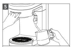
Press ▶I⊗ button to initiate the steam. Froth until desired level of foam and temperature is reached. To stop the steam, press ▶I⊗ button again. To avoid splattering, wait until the steam stops before removing the Steam Wand from the milk.
