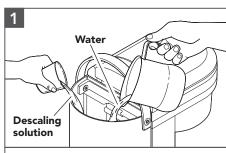
Fill 250 ml water and 125 ml descaling solution inside the Water Tank.
