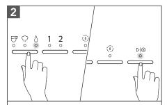
To change pre-programmed Water Hardness: Toggle the Mode Button to Water, Press and hold for 3 seconds. The indicator lights will show the default factory setting or previous saved setting (see Indicator light chart for reference). Toggle the Mode Button between Low-Mid-High to select desired water hardness. To save your selection, press ▶I❷ button or wait for 10 seconds.
