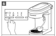
To rinse the Steam Wand, direct the Steam Wand towards the Drip Tray or into a cup. Then, toggle the Mode Button to select Hot Water and press ▶I⊗ button to start.
