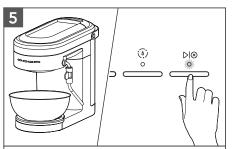
Phase 4: Place the container (~0.5 L) on the Drip Tray below Group Head. Then, press ▶1⊗ button. Clean ⑤ light and ▶1⊗ button light will blink fast after the fourth and final phase is complete. Empty the container.
