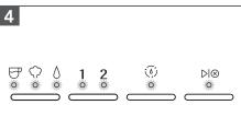
The machine automatically pumps water into the heater and starts heating. When lights stop blinking, the Espresso Machine is ready for use.
