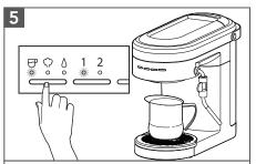
To rinse the Group Head, place a container under the Group Head. Toggle the Mode Button to select Espresso. Toggle Dose Button to 1 and press DO button. The machine will flush water through the Group Head and automatically stop when the cycle is complete.
