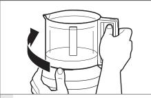
Hold the base steady with one hand, and use the other hand to rotate the work bowl clockwise to unlock and lift it off of the base.
