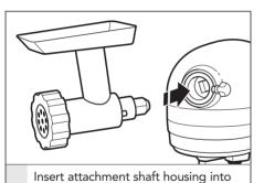
attachment hub, making certain that attachment power shaft fits into square attachment hub socket. It may 3 be necessary to rotate attachment back and forth. When attachment is in proper position, the pin on the attachment will fit into the notch on the hub rim.
