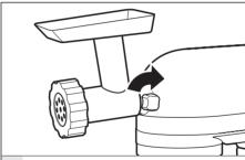
Tighten attachment knob by turning 4 clockwise until attachment is completely secured to Stand Mixer.
