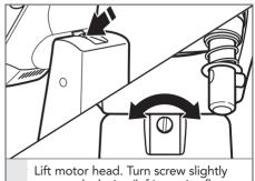
counterclockwise (left) to raise flat beater or clockwise (right) to lower flat beater. Make adjustment with flat beater, so it just clears surface of bowl. If you over adjust the screw. the bowl lock lever may not lock into place.
