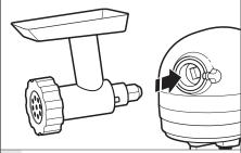
Insert attachment shaft housing into attachment hub, making certain that attachment power shaft fits into square attachment hub socket. It may be necessary to rotate attachment back and forth. When attachment is in proper position, the pin on the attachment will fit into the notch on the hub rim.
