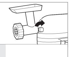
4 Tighten attachment knob by turning clockwise until attachment is completely secured to Stand Mixer.
