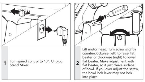
**NOTE:** When properly adjusted, the flat beater will not strike on the bottom or side of the bowl. If the flat beater or the wire whip is so close that it strikes the bottom of the bowl, coating may wear off the beater or wires on whip may wear.
