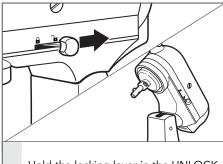
**2** Hold the locking lever in the UNLOCK position and tilt motor head back.
