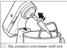
3 press upward as far as possible. Then, turn accessory to the right, hooking accessory over the pin on the shaft.
