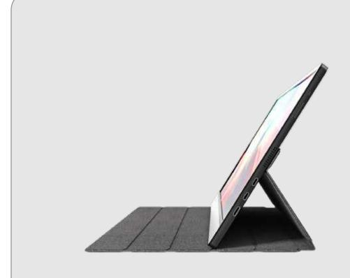
Placement 3: Adjustable 69.35±3° with the horizontal plane
