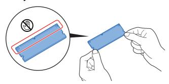
To protect electronic parts, discharge static electricity from your body by wearing an antistatic wrist strap, if possible, when you install the memory modules. If you do not have a wristband, touch a metal object to discharge static electricity before inserting the memory.
