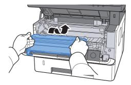
Return the developer unit together with the toner container to its position, aligning the guides at both ends with the slots in the machine.
