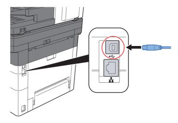
2 Connect the other end of the cable to the PC.
