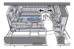
7 On the drum unit, slide the main charger cleaner back and forth 2 or 3 times to clean the charger wire.
