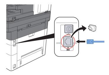
2 Connect the other end of the cable to the hub or the PC.
