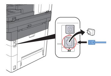
2 Connect the other end of the cable to the hub or the PC.
