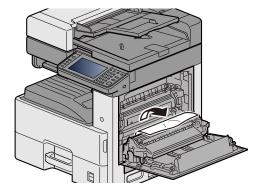
3 Open the fuser cover (a) and remove any jammed paper.
