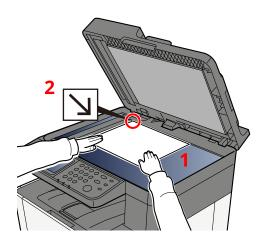
2 Align it flat against the original size indicator plates with the back left corner as the reference point.
