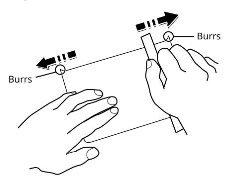
Before loading Hagaki (Cardstock) into the multipurpose tray, fan them and align the edges. If the Hagaki (Cardstock) paper is curled, straighten it before loading. Printing onto curled Hagaki (Cardstock) may cause jams.
