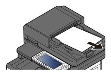
Open the Document Processor cover and remove the jammed paper.
