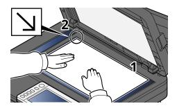
2 Align it flush against the original size indicator plates with the back left corner as the reference point.
