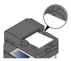
Ensure that loaded originals do not exceed the level indicator. Exceeding the maximum level may cause the originals to jam.
