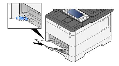
Insert the paper along the paper width guides into the tray until it stops.
