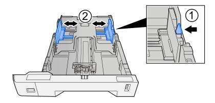
2 Adjust the paper length guide to the paper size required. Press the paper length adjusting tab and slide the guides to the paper size required.
