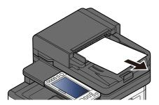
**7** Open the Document Processor cover and remove the jammed paper.
