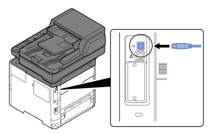
2 Connect the other end of the cable to the PC.
