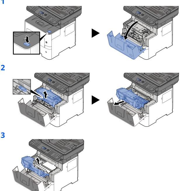
If the jammed paper appears to be pinched by rollers, pull it along the normal running direction of the paper. If you cannot find a paper jam, try checking inside the rear of the printer.
