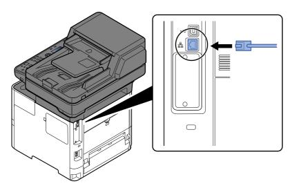
**2** Connect the other end of the cable to the hub.
