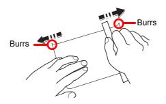
Before loading Hagaki (Cardstock) into the multipurpose tray, fan them and align the edges. If the Hagaki (Cardstock) paper is curled, straighten it before loading. Printing onto curled Hagaki (Cardstock) may cause jams.
