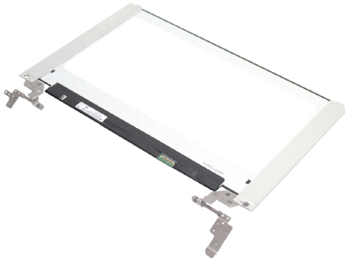
Figure 68. Remove the LCD assembly
