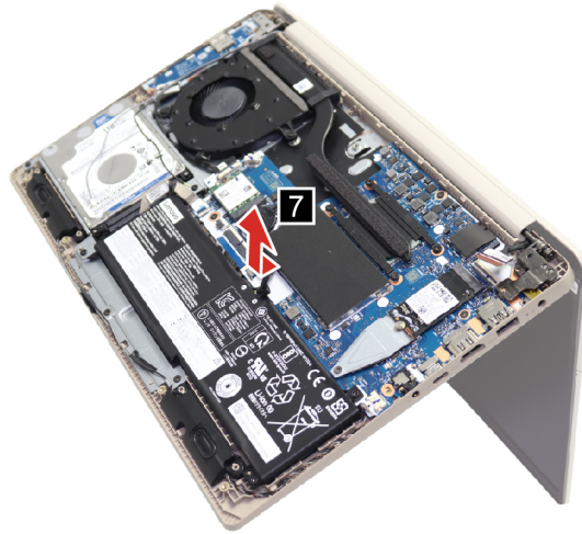
Figure 57. Remove the upper case assembly
