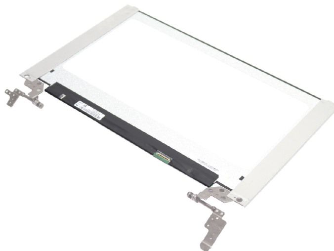
Figure 68. Remove the LCD assembly
