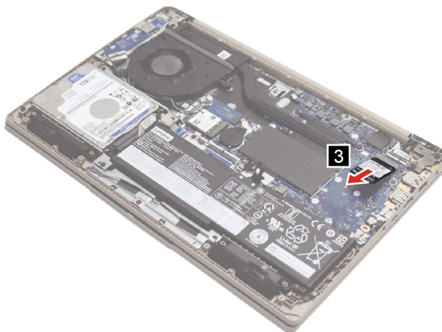
Figure 19. Remove the solid-state drive
