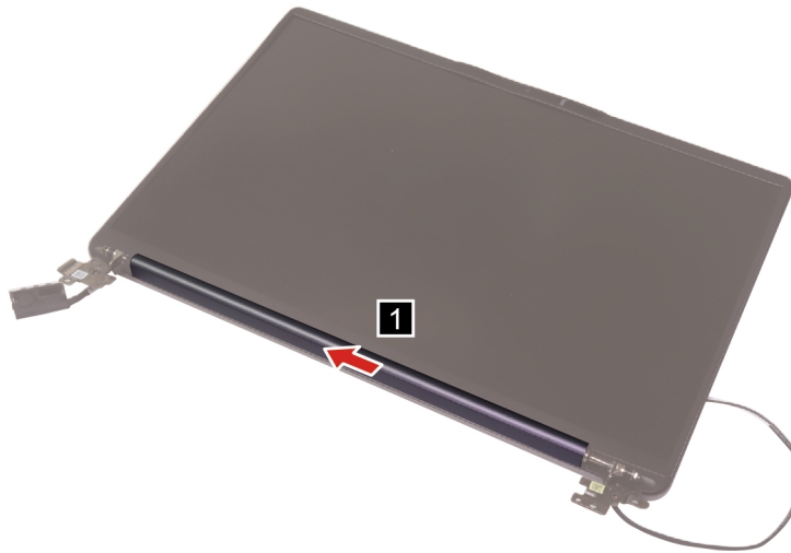
Figure 41. Slide the hinge cover to left side and remove the hinge cover
