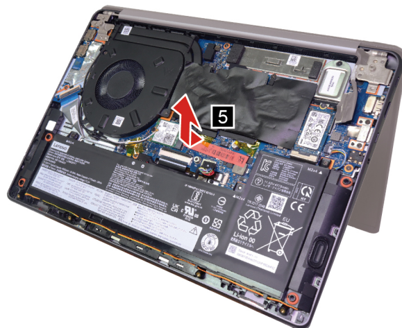
Figure 40. Remove the upper case assembly
