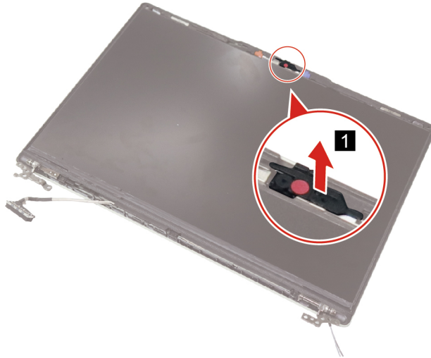
Figure 48. Remove the camera shutter
