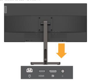
Connect one end of the HDMI cable to the monitor HDMI connector and the other end to the computer.
