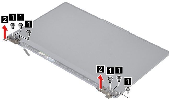
Figure 34. Remove the hinge
