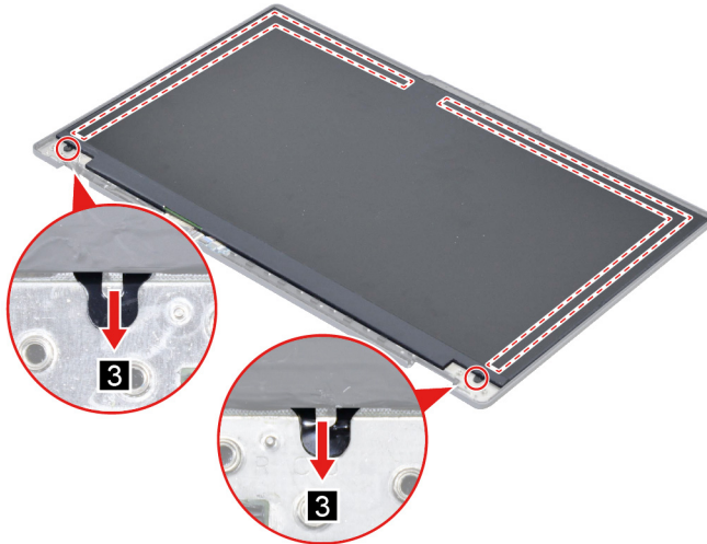
Figure 35. Remove the two pieces of removable tape
