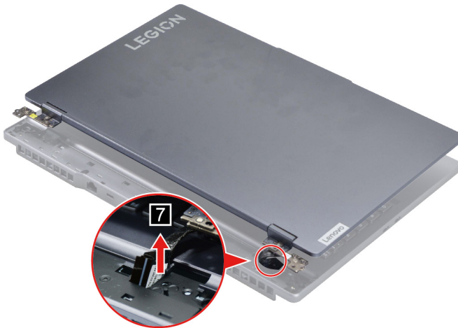
Figure 31. Take out the EDP cable and then remove the LCD module
