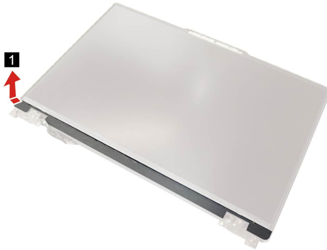
Figure 32. Remove the hinge cover
