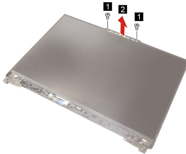
Figure 34. Remove two screws and remove the camera bracket
