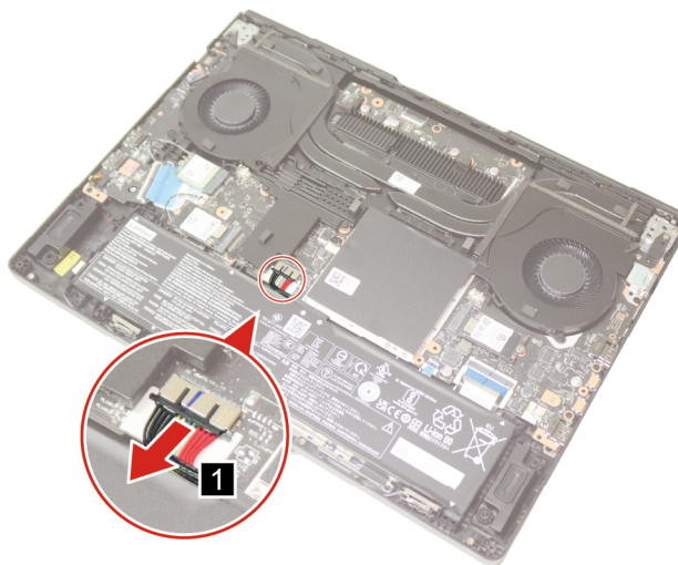
Figure 14. Disconnect the battery pack cable
