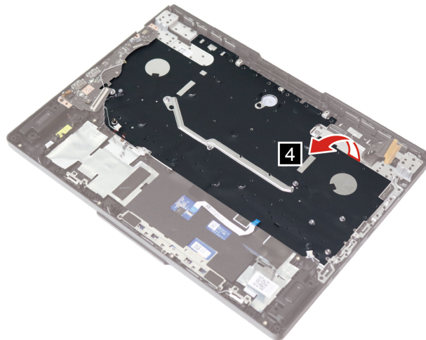
Figure 34. Peel back the protective mylar
