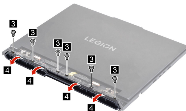
Figure 28. Remove the rear lightingbar
