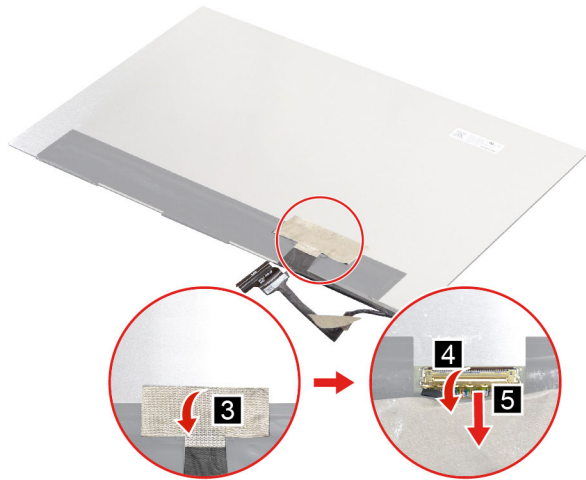
Figure 51. Remove the EDP cable
