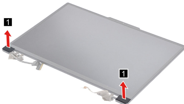
Figure 48. Remove the hinge cap
