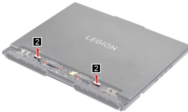
Figure 38. Remove the antenna
