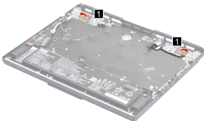
Figure 39. Peel off the two pieces of tape
