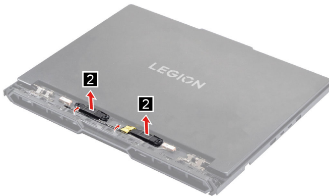
Figure 26. Remove the speakers
