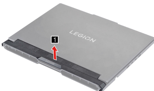
Figure 7. Remove the strip cover
