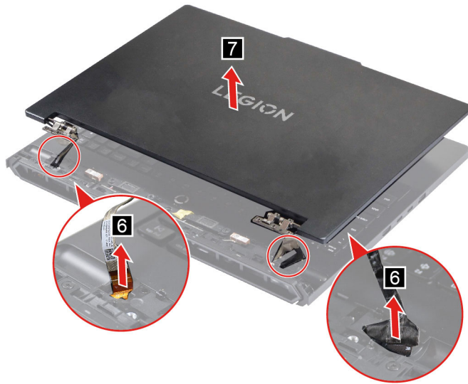
Figure 42. Remove the LCD module
