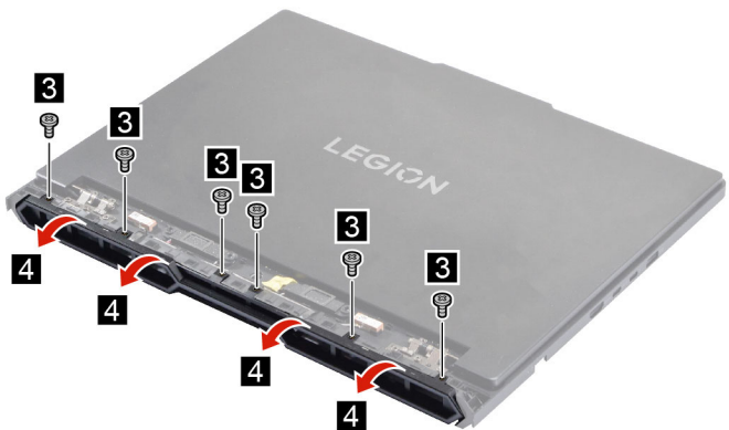
Figure 32. Remove the rear lightingbar
