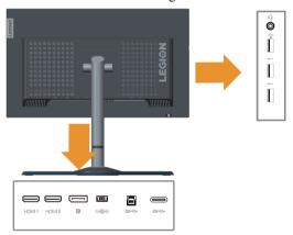
3. Connect one end of the DP cable to the DP connector on the back of the computer, and the other end to the DP connector on the monitor. Lenovo recommends that customers who require to use the Display Port input on their monitor purchase the "Lenovo Display Port to Display Port cable 0A36537". www.lenovo.com/support/monitoraccessories
