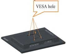
Step 5: Attach the LCD display to the wall, and follow the instructions in the wall-mounting kit. For use only with UL Listed Wall Mount Bracket with minimum weight/load: 8kg
