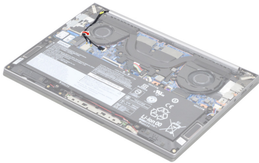
Figure 15. Release the antenna cable from the cable guide
