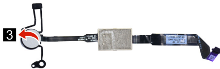
Figure 69. Remove the switch cover
