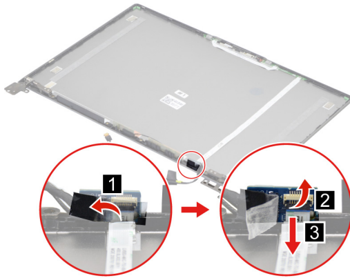
Figure 48. Peel off the tape and then disconnect the camera cable from the trans board
