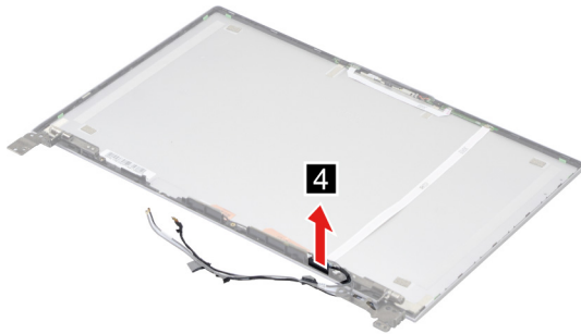
Figure 100. Remove the trans board with cable
