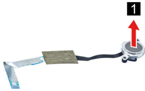
Figure 72. Remove the fingerprint board lens light guide
