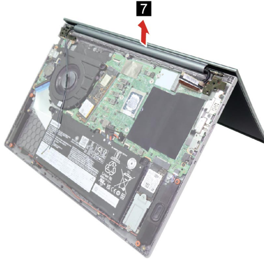
Figure 36. Rotate and remove LCD module
