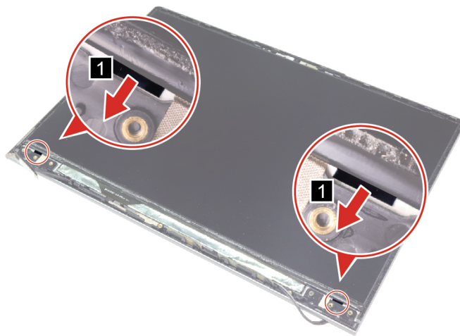
Figure 41. Use tweezers to pull out the adhesive tapes
