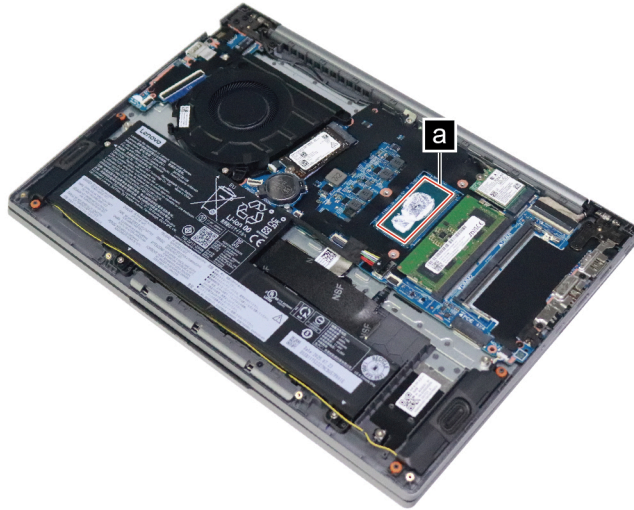
Figure 19. Area on the system board where thermal interface materials are applied
