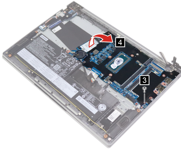
Figure 32. Remove one screw and remove the system board
