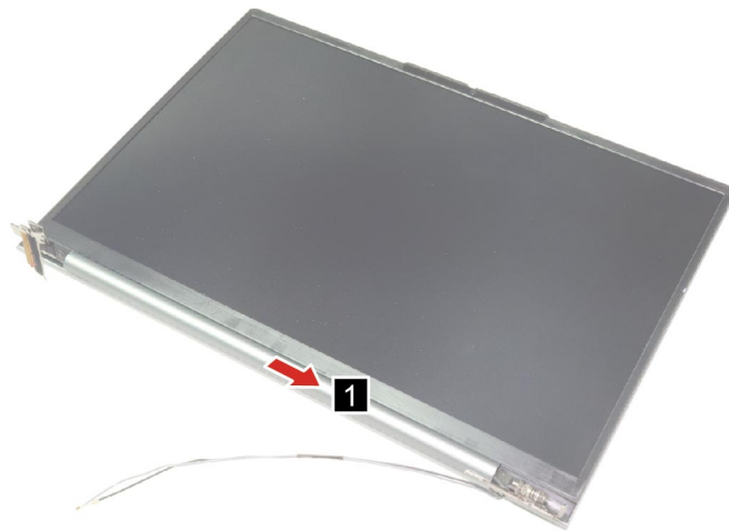
Figure 39. Remove the hinge cover
