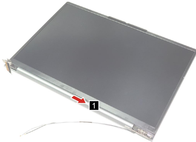
Figure 38. Remove the hinge cover
