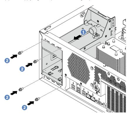
Figure 123. Hot-swap power supply cage installation
