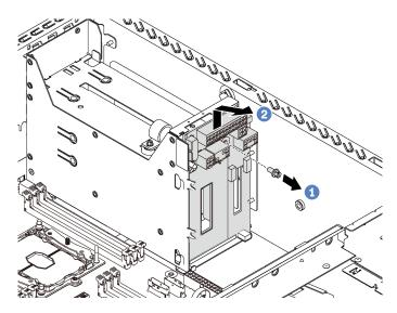
Figure 120. Power interface board removal
