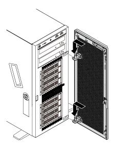
Figure 40. Front door installation
