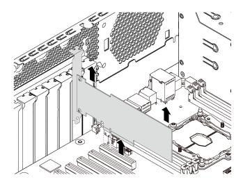
Figure 94. PCIe adapter removal
