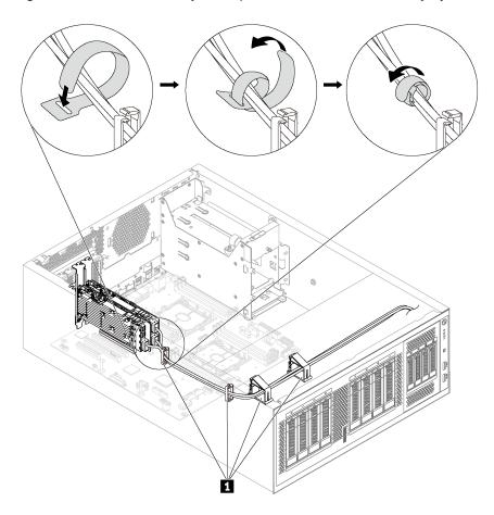
Figure 88. Securing and binding the signal cables correctly
