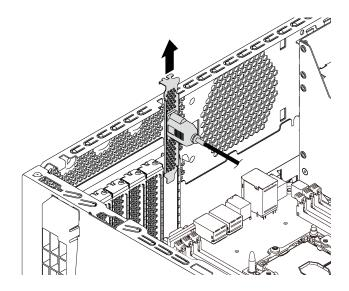
Figure 98. Serial port module removal
