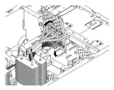
Figure 79. Simple-swap-drive backplate installation
