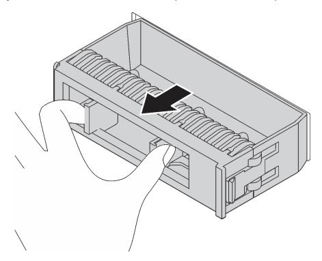
Figure 72. 3.5-inch drive filler removal
