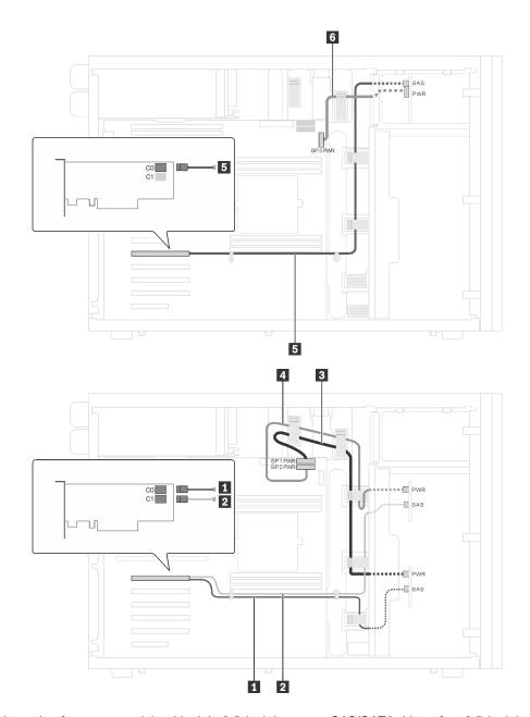
Figure 35. Cable routing for server models with eight 3.5-inch hot-swap SAS/SATA drives, four 2.5-inch hot-swap SAS/SATA drives, and two 8i RAID adapters
