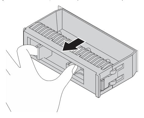
Figure 76. Drive filler removal
