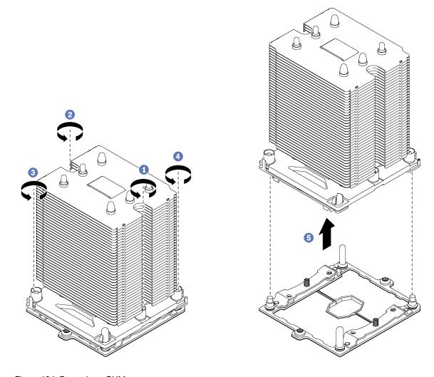
Figure 124. Removing a PHM
