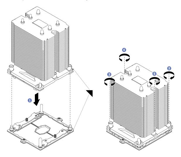
Figure 130. Installing a PHM
