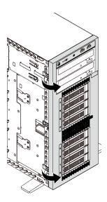
Figure 57. Front bezel removal
