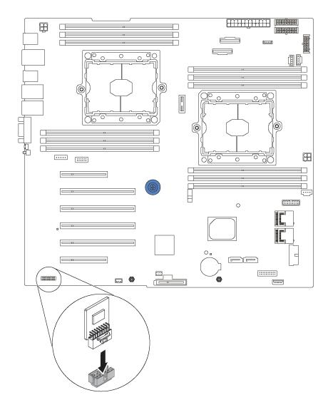
Figure 108. TCM/TPM adapter installation
