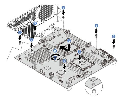
Figure 132. System board installation
