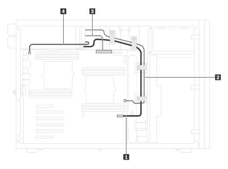
Figure 16. Cable routing for the power interface board
