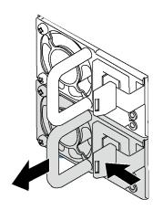
Figure 116. Hot-swap power supply removal
