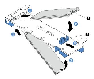
Figure 104. M.2 drive installation
