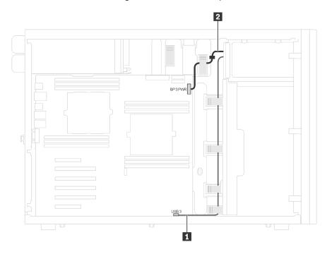
Figure 15. Cable routing for the USB tape drive
