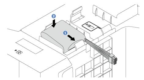
Figure 48. RAID super capacitor module installation
