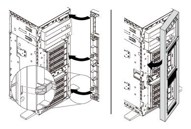
Figure 58. Front bezel installation
