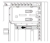
Figure 67. Drive retainer removal
