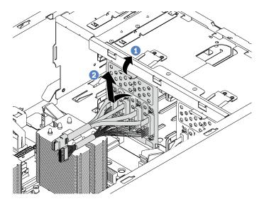
Figure 78. Simple-swap-drive backplate removal
