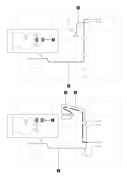
Figure 37. Cable routing for server models with eight 3.5-inch hot-swap SAS/SATA drives, four 2.5-inch hot-swap SAS/SATA drives, and one 32i RAID adapter
