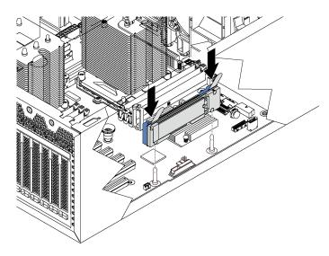
Figure 106. M.2 backplane installation
