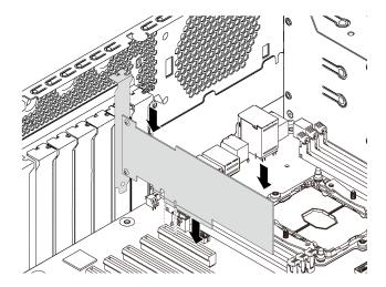
Figure 95. PCIe adapter installation
