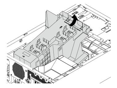
Figure 49. Air baffle removal
