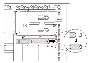
Figure 64. Drive retainer installation
