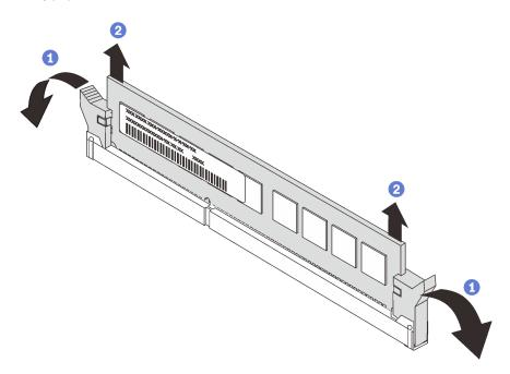
Figure 89. DIMM removal
