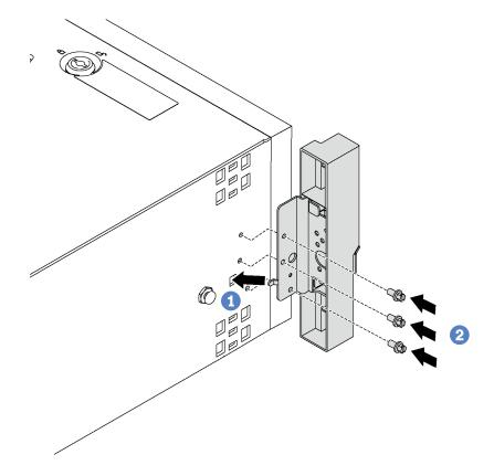
Figure 44. Rack latch installation
