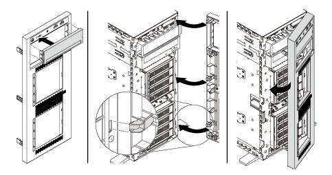
Figure 63. Drive-bay-filler cover installation
