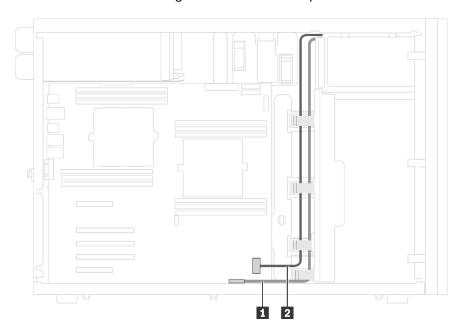
Figure 12. Cable routing for the front panel
