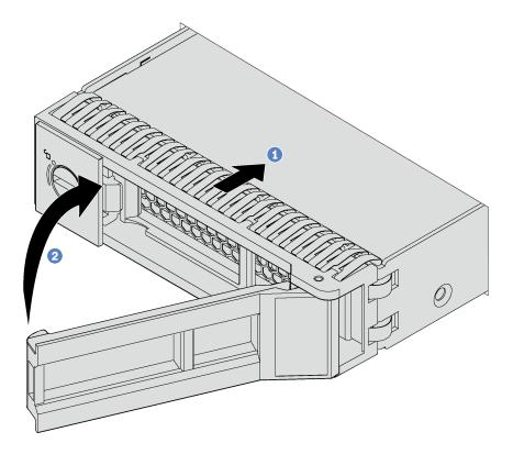
Figure 73. 3.5-inch simple-swap drive installation
