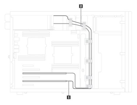
Figure 18. Cable routing for the graphics adapters
