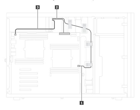
Figure 17. Cable routing for the fixed power supply
