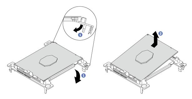
Figure 126. Removing a processor retainer
