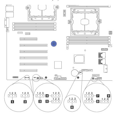
Figure 11. System board jumpers
