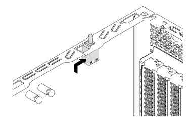
Figure 110. Intrusion switch installation
