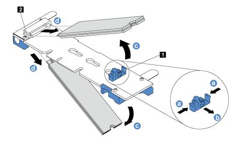
Figure 101. M.2 drive removal
