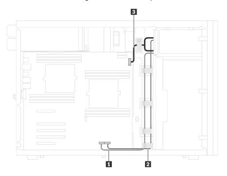
Figure 13. Cable routing for the optical drives
