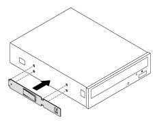
Figure 68. Optical drive retainer installation
