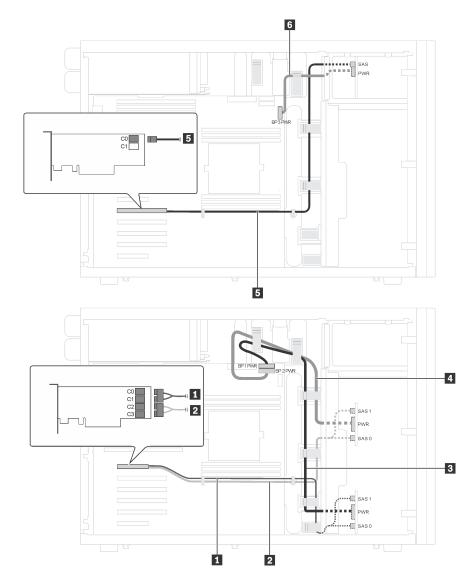
Figure 30. Cable routing for server models with twenty 2.5-inch SAS/SATA drives, one 8i RAID adapter and one 16i RAID adapter
