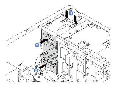
Figure 86. Expansion drive cage removal
