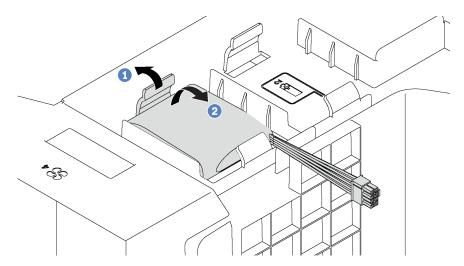
Figure 47. RAID super capacitor module removal
