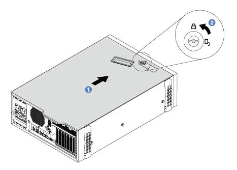
Figure 46. Server cover installation
