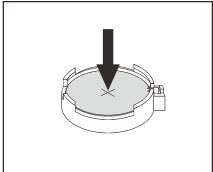
Figure 97. CMOS battery installation
