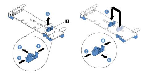
Figure 102. M.2 retainer adjustment
