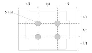
Figure 128. Proper shape of the thermal grease
