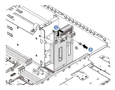
Figure 121. Power interface board installation
