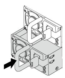
Figure 119. Hot-swap power supply installation
