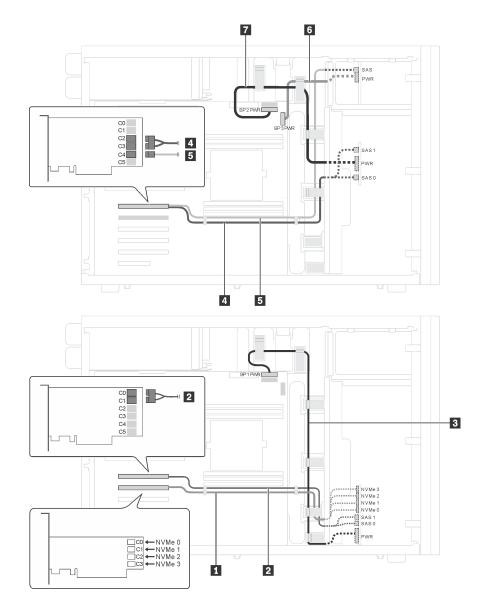
Figure 31. Cable routing for server models with sixteen 2.5-inch SAS/SATA drives, four 2.5-inch SAS/SATA/NVMe drives, one 24i RAID adapter, and one NVMe adapter
