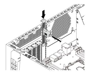
Figure 99. Serial port module installation
