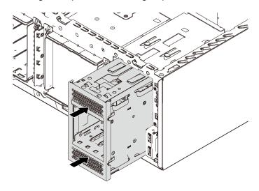
Figure 87. Expansion drive cage installation
