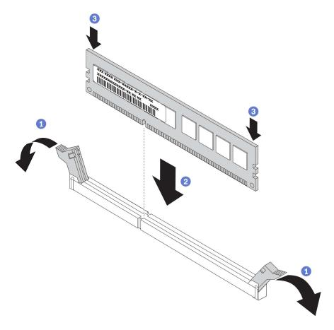
Figure 91. DIMM installation
