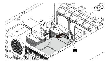
Figure 92. PCIe adapter retainer removal
