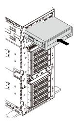
Figure 69. Optical drive installation
