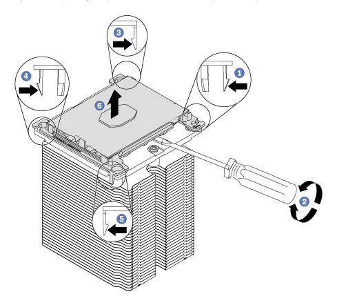
Figure 125. Separating a heat sink from a processor
