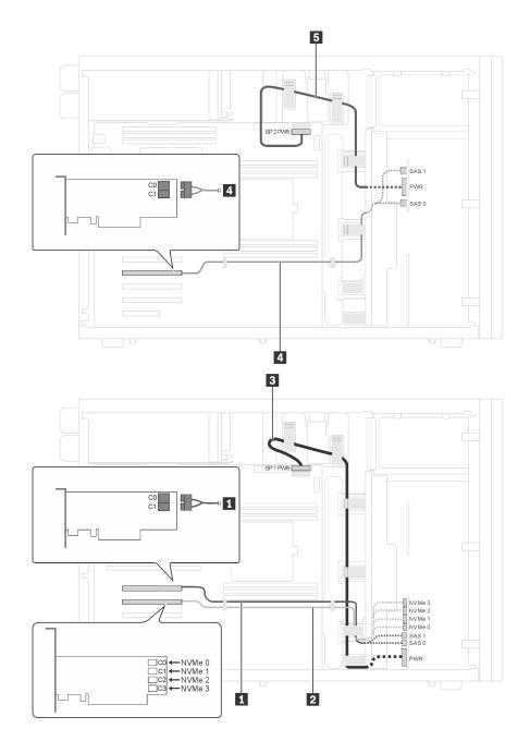
Figure 27. Cable routing for server models with twelve 2.5-inch SAS/SATA drives, four 2.5-inch SAS/SATA/NVMe drives, two 8i RAID adapters, and one NVMe adapter
