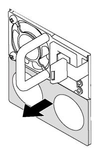
Figure 118. Hot-swap power supply filler removal
