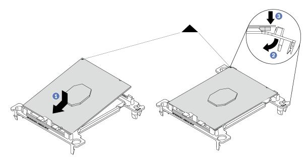
Figure 127. Installing a processor retainer
