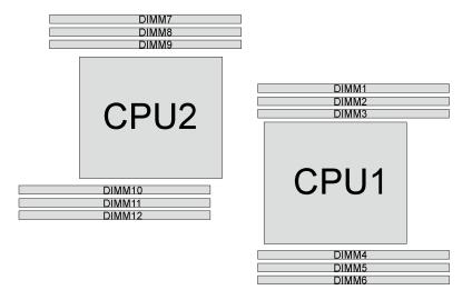
Figure 90. DIMM slots on the system board
