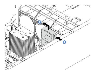
Figure 55. PCIe adapter holder removal
