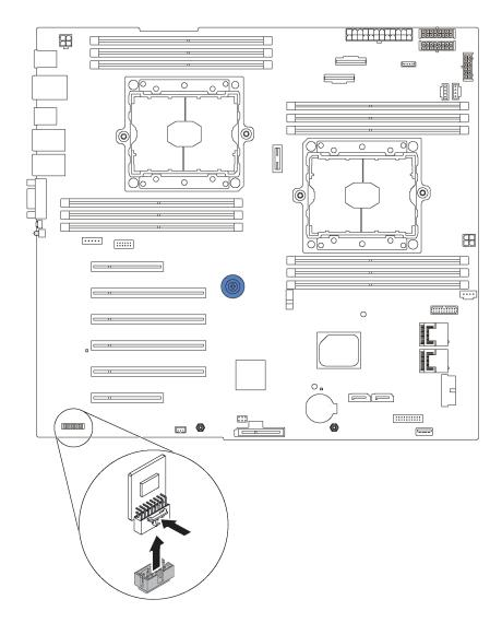
Figure 107. TCM/TPM adapter removal
