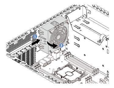
Figure 53. Rear fan removal
