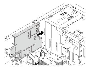
Figure 60. Front panel installation
