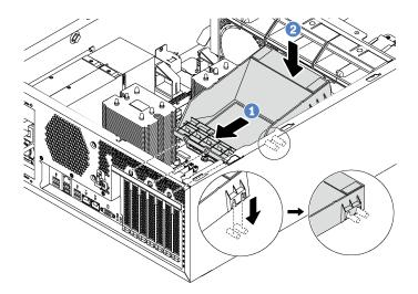
Figure 93. PCIe adapter retainer installation
