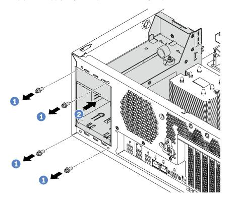
Figure 122. Hot-swap power supply cage removal
