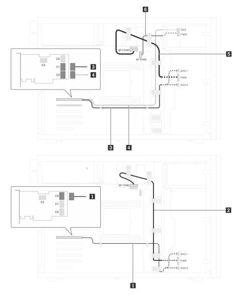
Figure 29. Cable routing for server models with twenty 2.5-inch SAS/SATA drives and one 32i RAID adapter
