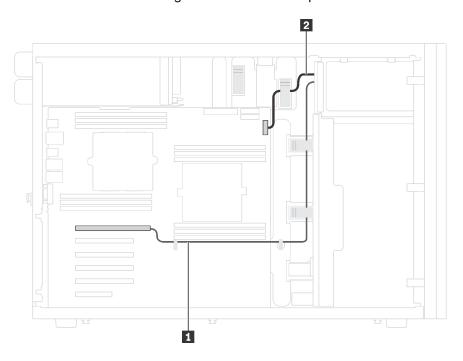
Figure 14. Cable routing for the SAS tape drive
