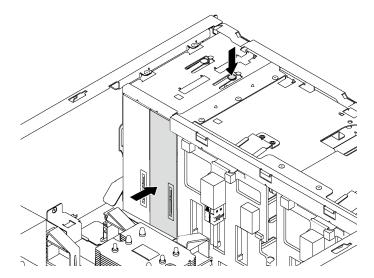
Figure 61. Optical drive removal
