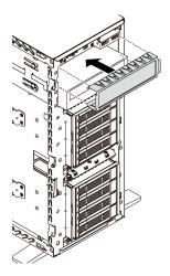
Figure 62. Drive bay filler installation
