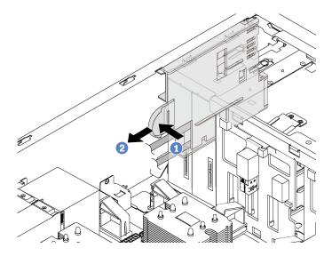
Figure 59. Front panel removal
