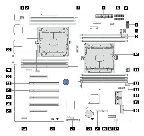
Figure 10. System board components
