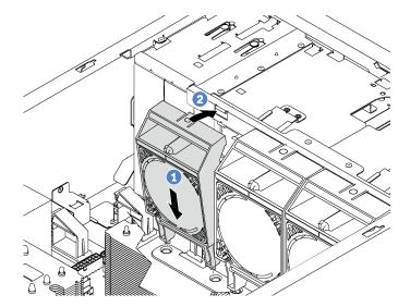
Figure 52. Front fan installation
