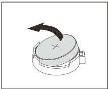
Figure 96. CMOS battery removal
