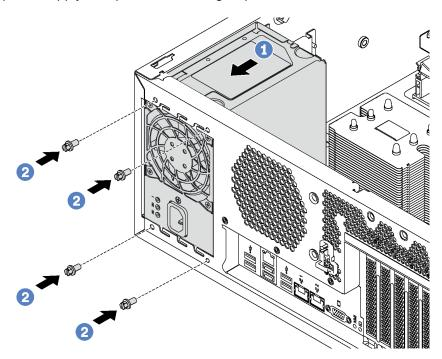
Figure 114. Fixed power supply installation
