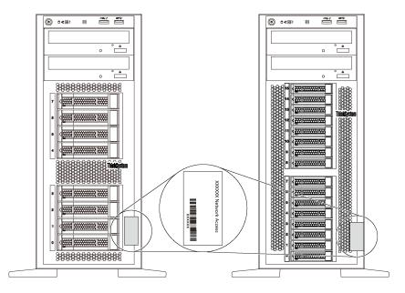
Figure 2. Location of the XClarity Controller network access label
