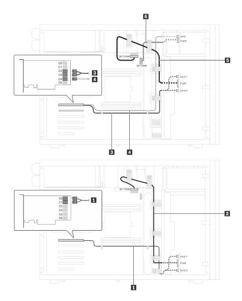
Figure 28. Cable routing for server models with twenty 2.5-inch SAS/SATA drives and one 24i RAID adapter
