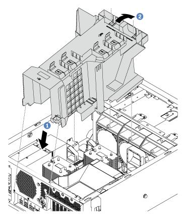
Figure 50. Air baffle installation
