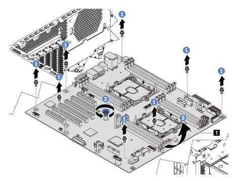
Figure 131. System board removal
