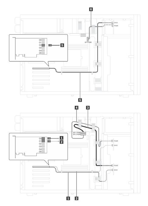
Figure 36. Cable routing for server models with eight 3.5-inch hot-swap SAS/SATA drives, four 2.5-inch hot-swap SAS/SATA drives, and one 24i RAID adapter
