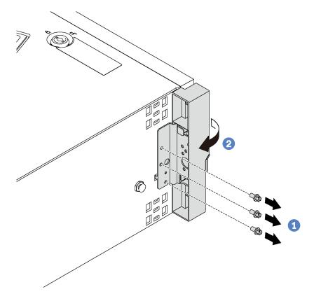
Figure 43. Rack latch removal
