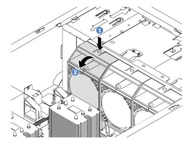
Figure 51. Front fan removal
