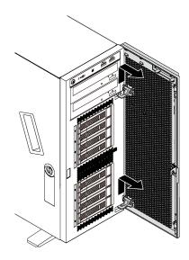
Figure 39. Front door removal
