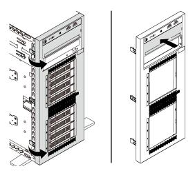
Figure 65. Drive-bay-filler cover removal
