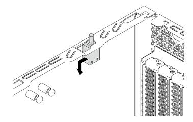
Figure 109. Intrusion switch removal
