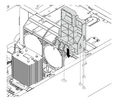
Figure 56. PCIe adapter holder installation
