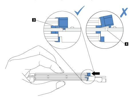
Figure 105. Instruction for sliding the retainer
