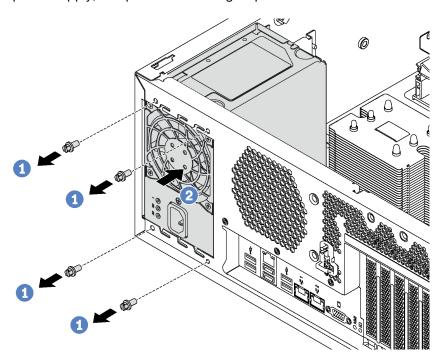
Figure 112. Fixed power supply removal
