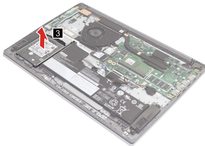
Figure 10. Disconnect the storage drive cable and remove the storage drive with bracket
