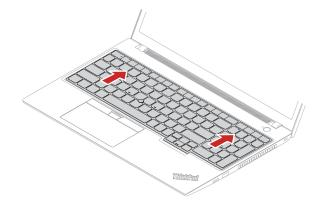
3. Pivot the keyboard slightly upward **II** and then turn over the keyboard **II**.
