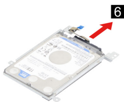
Figure 9. Remove the HDD cable
