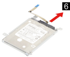
Figure 44. Remove the HDD cable
