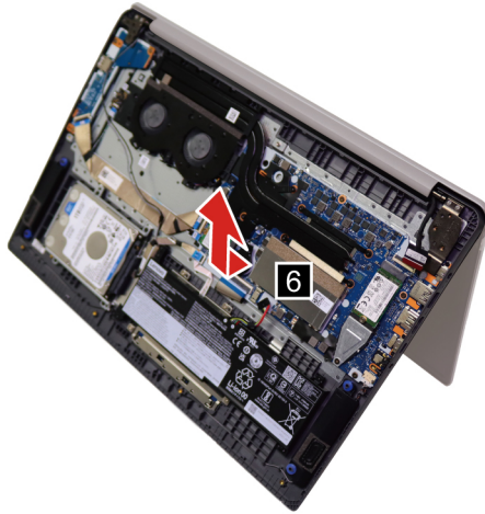
Figure 38. Remove the LCD unit
