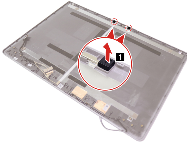
Figure 43. Remove the microphone rubbers
