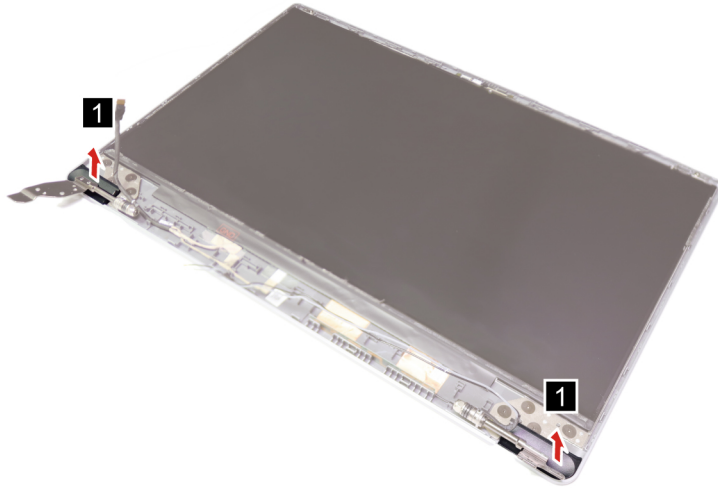
Figure 40. Remove the hinge covers
