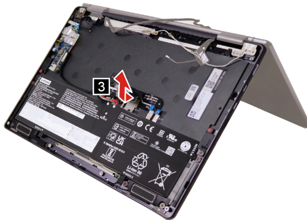
Figure 38. Remove the upper case (with keyboard)
