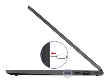
Step 2. Insert the SIM card in the SIM card tray. Note the orientation of the card and ensure that it is seated correctly.
