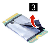
Figure 11. Separate the SSD mylar from the SSD
