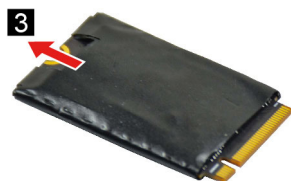
Figure 13. Remove the SSD foil from the SSD
