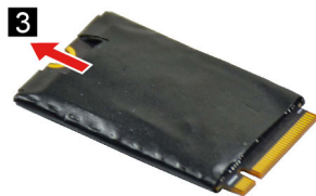
Figure 13. Remove the SSD foil from the SSD
