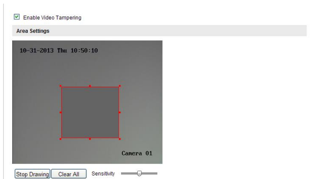
Figure 6-49 Video Tampering Alarm
