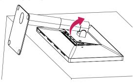
4 Pull the stand away from the monitor in its rotated position.
