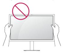
• Be careful not to touch or press the screen area when adjusting the angle of the monitor.
