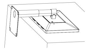
2 Push the Detach button on the back of the monitor to the left.
