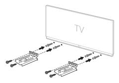
7 Place the product on the brackets. Position the product on the brackets so the screw holes on the bottom of the product align with the screw holes on the wall bracket.
