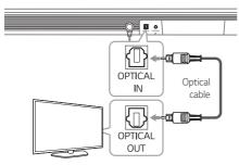
2. Select the input source to OPTICAL by pressing **F** button on the remote control or unit repeatedly.
