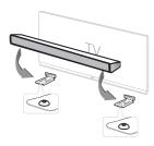
6. Fix the unit with the screws firmly.
