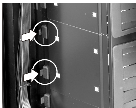
Press to release the HDD tray
